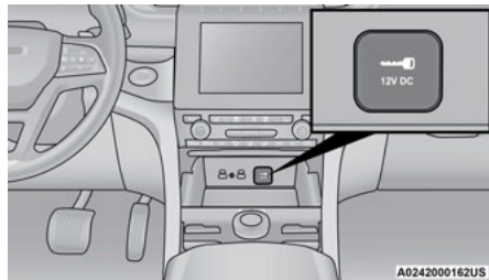
Front Power Outlet
